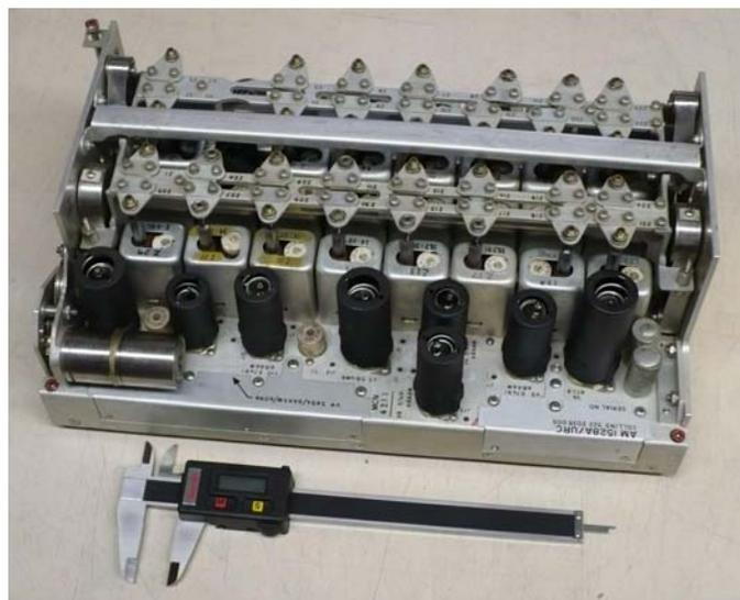
**Figure 3. AM-1528A RF tuner used in the ARC-58/TRC-75. The URC-32/KWT-6 tuner is similar but manually tuned**
